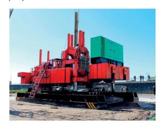
A pushing mechanism in the centre of the machine supplies the force to push the pile. This mechanism consists of a hydraulic clamp to hold the pile and four hydraulic cylinders providing a stroke of approximately 2m. The clamp can be adjusted for several round or square pile diameters or even piles of a different shape. The electric motors of the hydraulic pile pusher can be driven by a generator set or by any other electric power supply.
