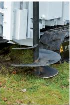
The Midi CPT Crawler consists of our proven HYSON 200 kN penetrometer mounted on an undercarriage with rubber tracks. The Midi CPT Crawler from A.P. van den Berg is designed to be compact, manoeuvrable and light, but with maximum power. With a weight of about 3,500 kilo and a width of only 1,200 mm the Midi CPT Crawler fits trough small passages and can be transported in a small truck. All these features ensure that the
